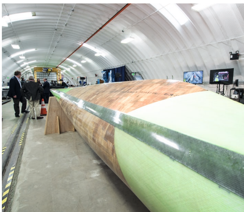
Wind turbine blades made of wood could make wind turbines more sustainable. Photo: Dennis Schroeder, NREL
