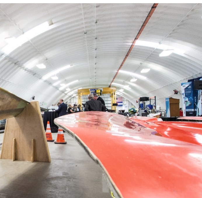
Wind turbine blades made of wood could make wind turbines more sustainable. Photo: Dennis Schroeder, NREL
